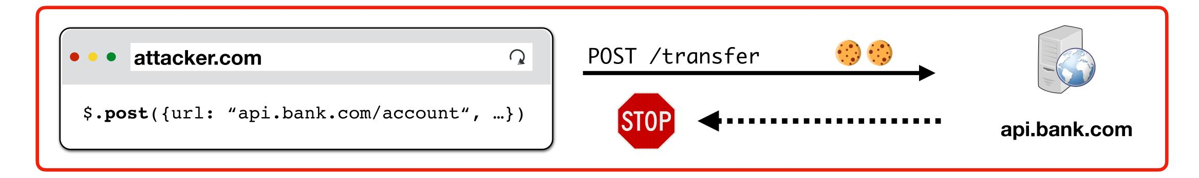
Cross-site request forgery (CSRF) attacks are a type of web exploit where a website transmits unauthorized commands as a user that the web app trusts
